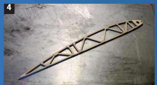
Method and step by step construction to make the framed up ribs
