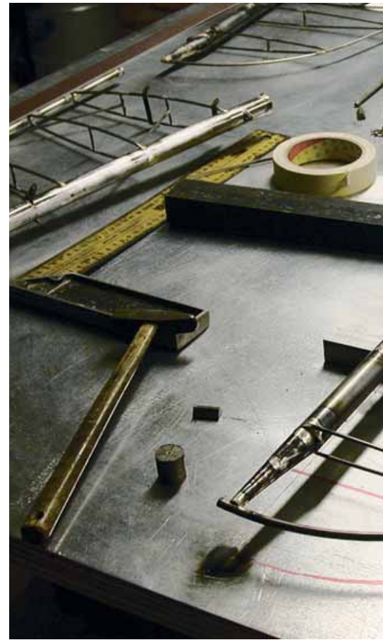
Above and below: construction of the tailplane with steel tube
